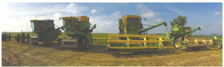
Iowa farmer Russ Bruhn collects vintage Deere combines. In total, he and his son and son-in-law have a Deere 45, a 55, four 95's, and two 105's. The 45 is the smallest, equipped with just a 2-row cornhead. The other machines can be fitted with a windrow pickup, a grain platform or a cornhead, all of which Bruhn has on hand.
