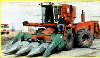
Vogel's rotary combine is longer and lower than conventional machines, due to its articulation. Vogel says it follows the row "like no other combine". The header, sieves, cab and discharge auger are the only parts salvaged from other combines.
