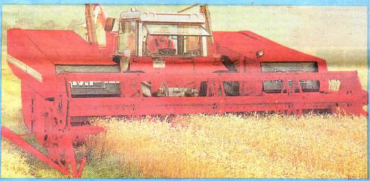
Massey's new combine, with field capacity comparable to biggest self-propelleds on market, divides grain swath in two as it's cut, running it through two separate but identical threshing units up either side of the tractor.
