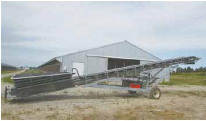
Portable 40-ft. long, 30-in. wide belt conveyor allows Ben Graber to load chicken litter into semi trucks fast.
