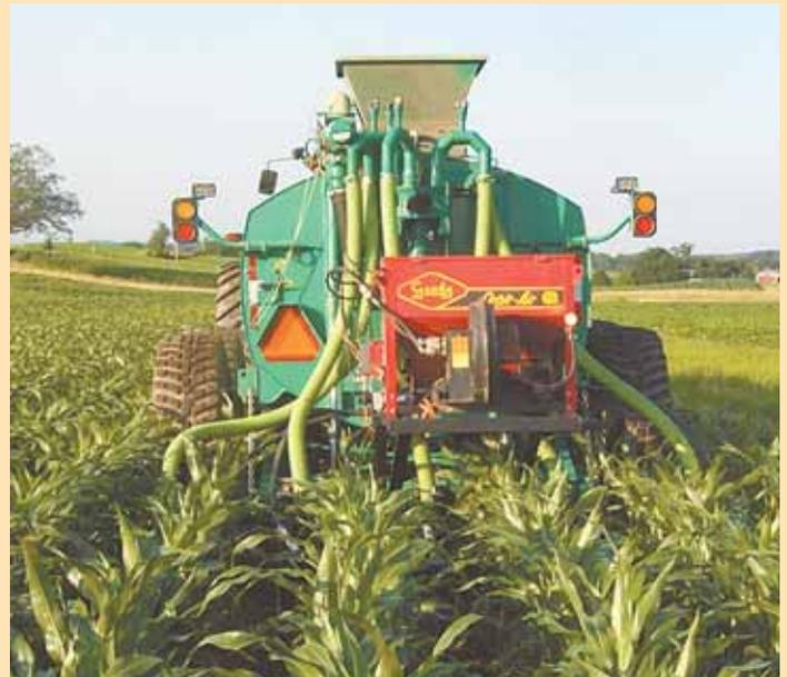
Liquid manure injection system sidedresses manure into standing corn. At the same time, a toolbar-mounted Gandy Orbit-Air seeder broadcasts cover crop seed.
