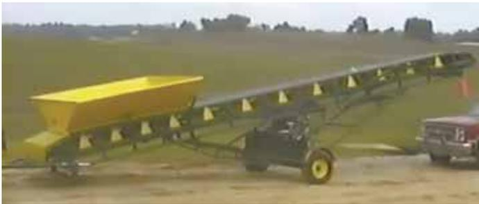
Richard Crabtree's home-built, 32-ft. conveyor loads manure into trucks about as fast as a skid loader can fill the hopper.
