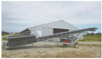
Portable 40-ft. long, 30-in. wide belt conveyor allows Ben Graber to load chicken litter
