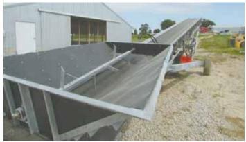
Variable speed motors drive a stirrator inside conveyor's hopper, and the belt.
