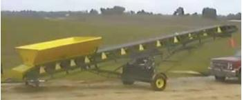
Richard Crabtree's home-built, 32-ft. conveyor loads manure into trucks about as fast as a skid loader can fill the hopper.
