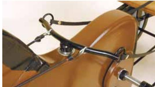
When a child sitting in cart pedals, legs on the wooden horse move. Pulling on the reins steers it. Photo at left shows how a T-bar above horse's back turns a wheel under horse as reins are pulled.
