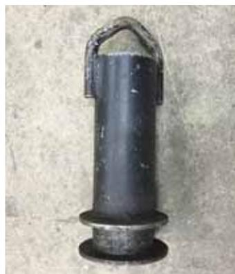
Homemade lift pin (left) and rolling storage rack makes it easier for Joe Campoli to handle his fifth wheel hitch. He inserts lift pin into hitch and uses an overhead hoist to install or remove hitch from pickup.
