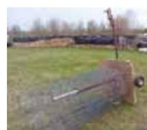
To load fence roll, Girard flips trailer on end so pipe is parallel to ground.
