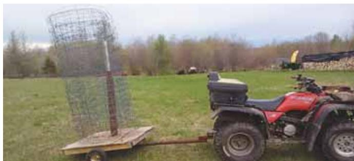
Atv-pulled, trailer-mounted fence unroller makes unwinding rolls of woven wire fencing an easy job for Roland Girard of Cochrane, Ontario.
