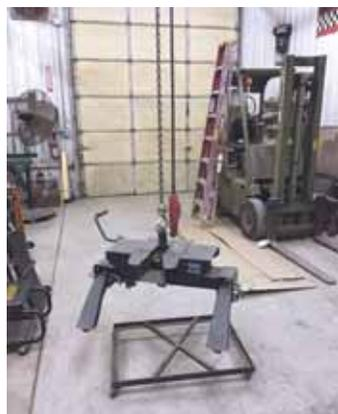
of the pipe. He bored out two 1 1/4-in. flat washers to fit the bottom of the pipe, then welded the washers in place leaving a 3/4-in. gap between them where the hitch locks on.
