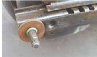
**Kurt Hofmeister, Woodburn, Oregon:** "Trying to assemble anything with loose washers often can be a frustrating experience. So if the washer is loose, I just roll a small O-ring onto the bolt and use it to hold the washer in place."
