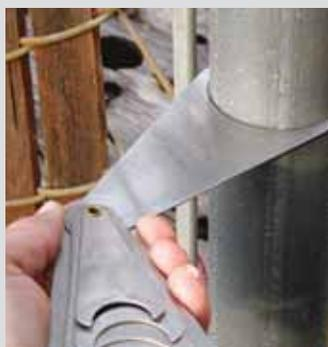
Tool consists of 7 riveted-together "sizers" that you fit over pipes to be measured.
