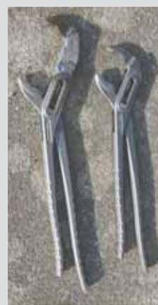
Andy Sewell extended the jaws on his channel lock pliers by cutting through jaw and welding in some steel.
