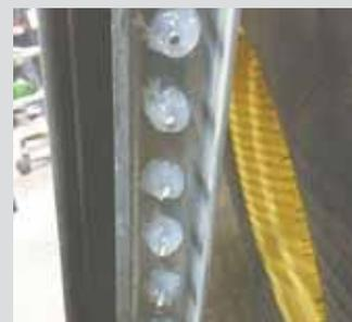
Photo shows worn sieve wires that Gutschmidt cut off with a Dremel tool. He welded new wire stock in place and then siliconed the ends to stop the wires from shaking.
