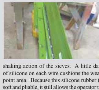
shaking action of the sieves. A little dab of silicone on each wire cushions the wear point area. Because this silicone rubber is soft and pliable, it still allows the operator to adjust the sieves. My sieves are adjustable from inside the cab with an electric actuator. The rubber gives enough to allow for the sieve to open and close all the way to adjust for any crop being harvested.”
