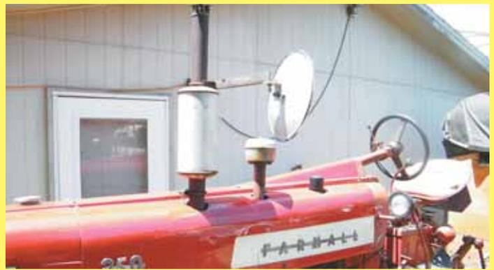
I mounted a mirror on the hood of an old yard tractor that we primarily use to move and spot trailers. Saves a lot of time lining up and it saves you from continually twisting to look back. It also helps keep an eye out for grandkids. Another tip is that I use a smaller 2-in. ball for hooking up to 2 5/16 ball hitches when moving trailers just a short distance. Makes it easier to connect. (Gary Swensen, Yankton, S. Dak.)
