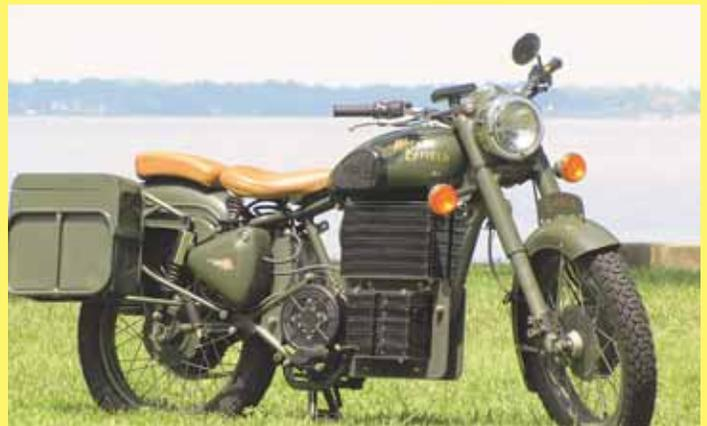
My Royal Enfield Bullet 500 motorcycle had a blown engine, so I had to do something. I decided to convert it to electric so it's now powered by a Motenergy ME1003 permanent magnet DC electric motor that goes where the transmission was and is located in front of the swing arm. Two stacks of batteries fill in the space where the engine used to be. They consist of 11 lithium battery modules taken from a Nissan Leaf electric car (the Leaf uses 48 modules).
