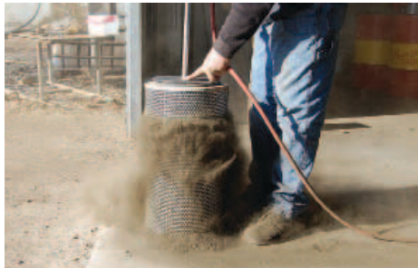
During tests on a pair of Deere 7750 tractors, one tractor’s air filter was cleaned once a day. Nearly 5 lbs. of dirt was removed daily and the tractor used 58 gal. less fuel per day than the tractor with the dirty filter.
