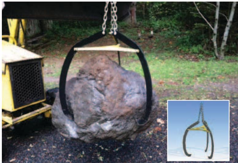
Rock Claw can handle big boulders with no problem. Three steel arms with curved points at their lower end are connected to a lift chain.
