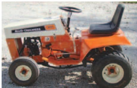
Tractor’s 5-speed transmission is operated by a Hurst car shifter located on one side of operator platform. Shifter is connected by a long metal rod to transmission’s shift linkage.
