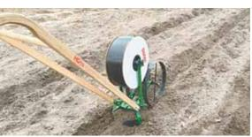
Hoss Tools's new drip irrigation tape layer attaches to the company's double wheel hoe, making it easy to lay down and bury drip tape in one pass.
