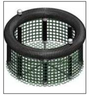
Underground watering system comes with a circular pvc reservoir that encircles the tree root ball. Water flows down towers into soaker hoses that form a criss-cross pattern at bottom of basket.
