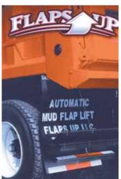
An electric motor control automatically raises mud flaps whenever truck is put in reverse. Driver pushes an in-cab switch to let flaps back down.
