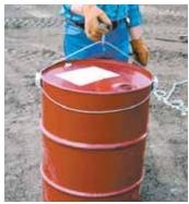
Brackets automatically lock in place under barrel rim as operator raises the unit.
