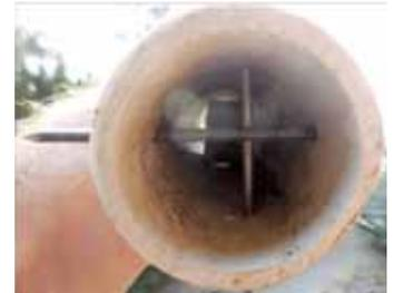
After shoving cubes into tube, Buelke inserts a pair of nails that crisscross the openings.
