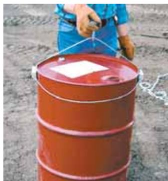
Brackets automatically lock in place under barrel rim as operator raises the unit.
