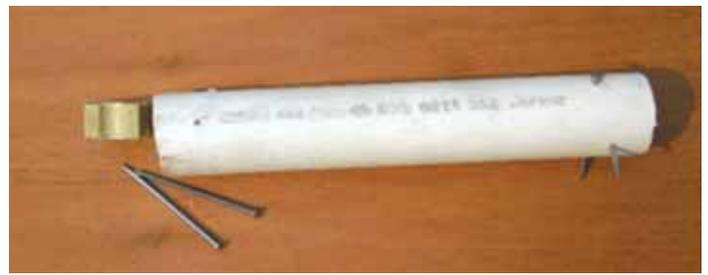
Don Buelke's high capacity mouse trap uses a short length of 1 1/2-in. dia. pvc tubing to hold poison cubes.
