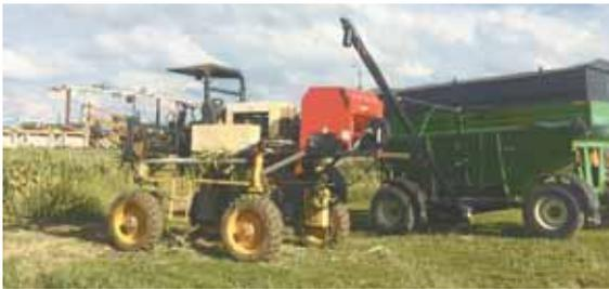
Modified detasseler spreads cover crop seed between corn rows, mulches it with chopped stalk tops, and opens up row centers for more light, all in one pass.
