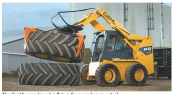
Tire Grabber can lay a tire flat on the ground or on a stack.
