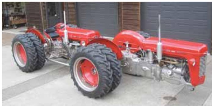
Lon Jackson built this MF-70 tandem tractor from two 1961 Massey Ferguson 35 models. A home-built “articulation pivot carrier” couples the tractors together.
