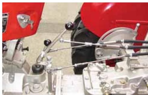
Controls between the 2 tractors are linked mechanically.
