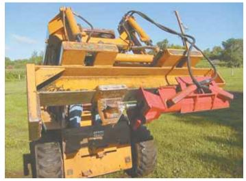
Mark Majerus made use of the auxiliary hydraulics on his Case skid loader to build this hands-free log splitter. It can be used as a "thumb" to pick up wood to split or load it onto a pile.
