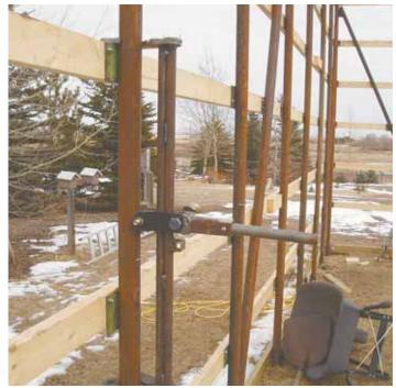
"Tensioner tool" works like a cam to slightly pre-bend pipe before McNaughton welds on it. It consists of a 3-ft. length of welded-together double pipes with steel hooks welded on top and bottom, and a pipe handle with a steel yoke at the end. (Photo illustrates use on pipe that has already been welded.)
