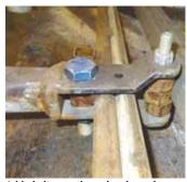
A big bolt runs through yoke and serves as a pivot point. Pulling down on handle causes another bolt with nuts on it to push against pipe to bend it inward.
