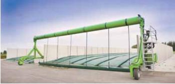
Retractable bunker cover system uses a set of A-frame gantries that run outside bunker walls, quickly unrolling or rolling up a weatherproof cover over silage. It's held in place by filling overlying hoses with water.
