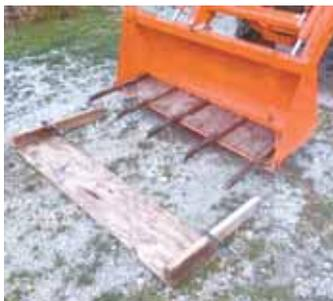
panels, and so on. When needed, I place a plywood platform over the forks to carry bulk items and use as a scaffold platform when working on buildings. I particularly like the loader’s hydraulic lock-out feature.”
