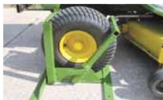
Operator raises a rear bracket up against tire and uses a set screw handle to tighten it in place.
