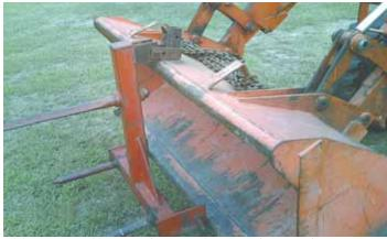
Williams welded a 6-in. length of square tubing on top of bucket to form a post, then bent a 2-in. strap iron to make a loop that bolts onto implement's top link.
