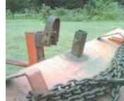
Bolt acts as a hinge and allows loop to be flipped up and over post.
