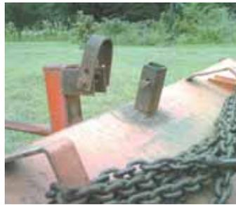
Bolt acts as a hinge and allows loop to be flipped up and over post.
