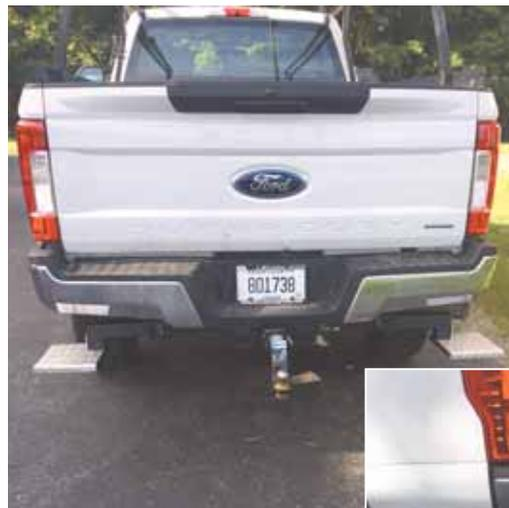
Add-on step slips into pickup’s receiver hitch. Lengths of square tubing support welded on steps on both sides of pickup.
