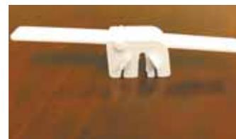
Mice will "walk the plank" to get to bait and fall into bucket. Trap then resets itself.
