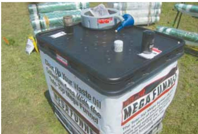
**Tote-Top Mega Funnel comes with a punched metal screen on top with a solid plastic layer beneath it that funnels drain oil down into tote for later disposal.**
