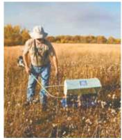
Hand-held seed harvester is powered by a heavy-duty line trimmer that operates parallel to the ground. It spins an 18-in. reel that grabs seeds and throws them into a hopper bag.
