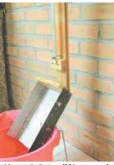
"Picker-upper" has a metal pan fastened to a hinge at the bottom. Whitmoyer pushes apples into pan with one foot and then pulls on handle to dump into a bucket.
