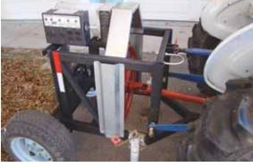
Don Prestien used the fan drive pulley and pto shaft off an old portable grain dryer to turn an old enginedriven, 10k generator into a pto-driven unit.
