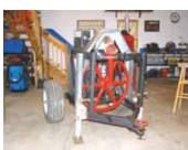
Generator mounts on a home-built 2-wheeled trailer (small pulley shown near fan drive pulley is not used to operate generator).
