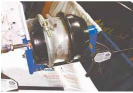
Klamp-It Brake Service Tool makes it easy for one person to change the brake diaphragms right on a truck.
