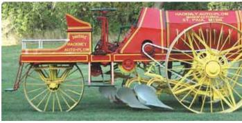
Rare 1912 Hackney One Man Auto Plow has a pair of lugged steel wheels on front and a single steel wheel on back. A 3 or 4-bottom moldboard plow mounts underneath.
