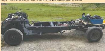
Winter cut the Prius unibody under the rear passenger seat and added a subframe (above). He then cut truck in two ahead of cab and overlaid the ends of the 2 frames. Removing the truck hood (right) reveals the Prius drive system.
