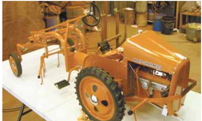
Allis Chalmers G pedal tractor is shown equipped with a cultivator. Other implements include a manure spreader, mower, harrow, turning plow, and planter.
