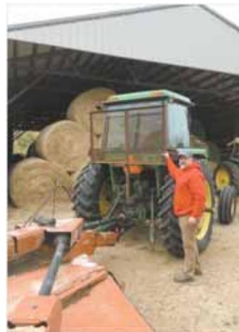
Expanded metal rock guard helps keep flying rocks from breaking tractor cab's rear window.
