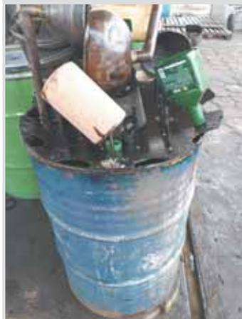
Plastic oil containers are placed over lengths of rebar welded to a big plow disc on top of barrel.
