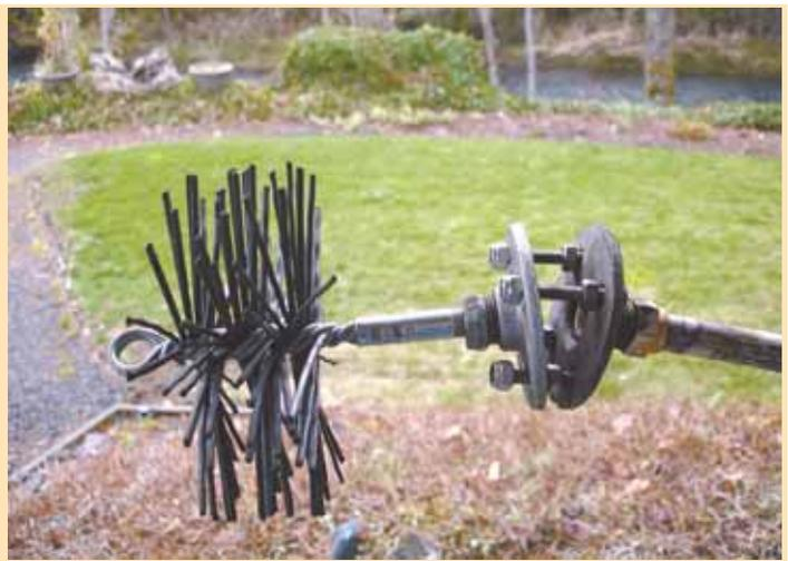
A pair of 1/2-in. thick galvanized flanges, connected loosely by 4 bolts, allow sweep to make a turn inside chimney.
