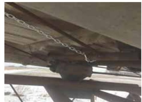
Up to 3 people can sit on the roomy, full-size pickup seat. The end drive gearbox off an old center pivot irrigator serves as the turntable mechanism for the cab.
