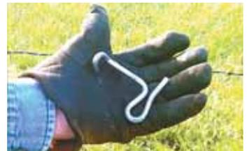
"This is the single most time and hassle-saving fence repair device that I've ever laid hands on. It consists of a clip that you wind into the fence wire with a crank handle. It won't break a barbed wire from bending it too sharp. You leave the clip in the fence, and later on you can grab the handle and give the clip another crank or two to retighten the wire, if necessary.
