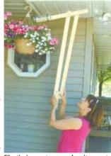
washers that allow them to pivot. One 4-ft. board remains stationary while the operator moves the other one up or down.
