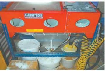
Andy Sewell came up with the idea of making a 3-handed sandblast cabinet, cutting up a second cabinet and adding half of it to his existing cabinet.
