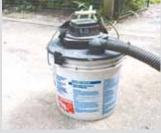
Mark Linda, Waterloo, Iowa: "When the metal body of my trusty old ShopVac rusted out, I got the idea of trying to fit the still-functioning vacuum onto the top of a plastic 5-gal. bucket. It was a perfect fit! The handle makes it easy to carry around."
