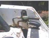
David Simpler, Elkton, Md.: "I needed a low-cost way to protect the hydraulic couplers on my skid loader, so I cut up an old heater hose that I already had into 3 to 4-in. lengths that friction fit onto the coupler. I used 1-in. hose for the male coupler and 1 3/8 in. hose for the female coupler. The hoses keep water out of the couplers. Works great.
