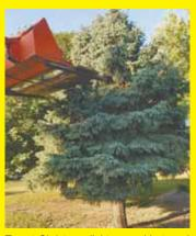
To put Christmas lights on a big tree, I made a platform for my loader bucket that installs in minutes with no bolts or other fasteners. It's held in place with a chain and come-along. I have pallet forks on the bucket and just slide them out to the sides of the bucket, and chain the platform in place. Works great. (Gary Swensen, Yankton, S.Dak.)
