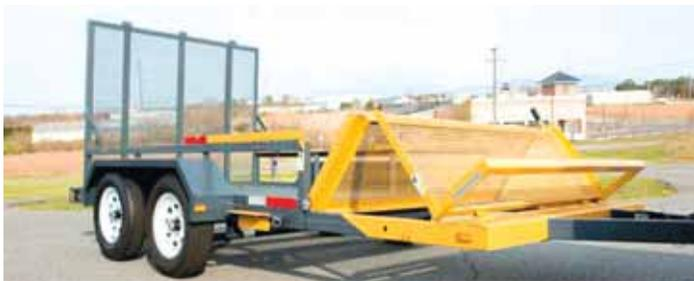
Trailer comes with a fold-up floor assembly on front - 2 pieces of expanded metal which are hinged in the middle and rest on a steel frame.
