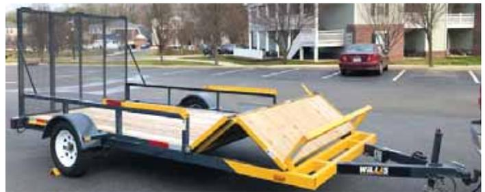
To return trailer to its original length, the operator uses a lever to break the plane on the extendable floor. He then applies the trailer brakes to lock the wheels, and backs up until trailer is compressed to its original length.
