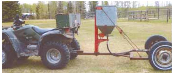
Dickinson mounted a Cyclone seeder on the wheels and axle off an old Toyota car. The axle’s differential is used to drive the seeder’s fan.
