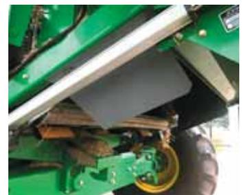
Kit attaches ahead of stalk chopper on Deere combines and drops crop residue in a 4-ft. wide strip for baling.
