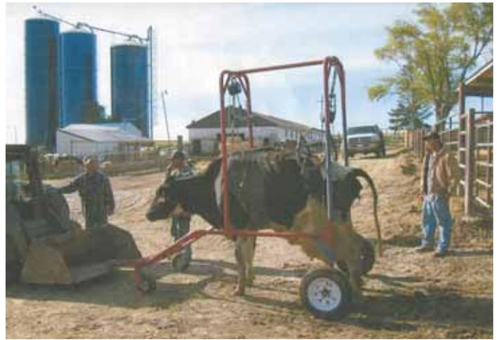
Wheeled sling lift is equipped with a nylon strap on front and a hip clamp on back, both operated by come-along hoists.
