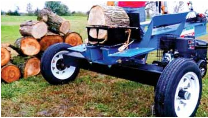
Home-built splitter can be used with 4 different splitting wedges that can be easily exchanged, as shown (below right).
