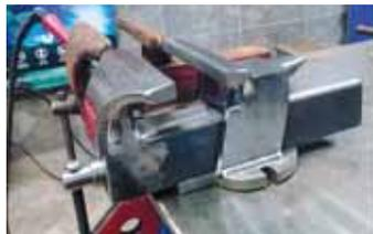
Metal spacers and magnets held jaws in place as he welded them to main vise frame.
