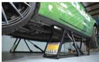
Electric-hydraulic portable car lift uses 2 frames to lift all 4 wheels off floor at the same time, and is operated by a remote control.
