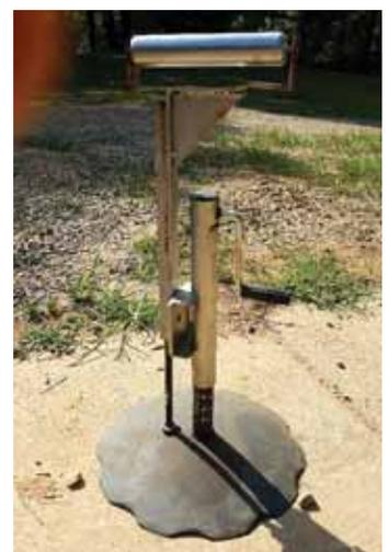
Johnson built several of these home-built trailer jack "roller stands", which he uses with his band saw to handle long material.
