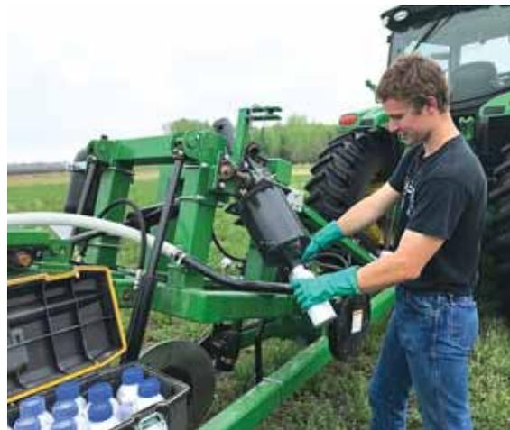
Pull-type machine uses a torpedo-shaped shank and a fan to deliver fumigant tablets into newly formed tunnels, gassing gophers to death.
