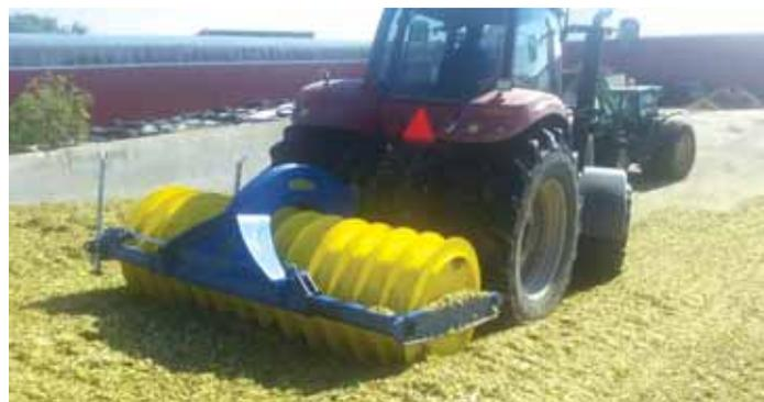
Roller's 4-in. tall fins provide concentrated compression, forcing air out of silage.
