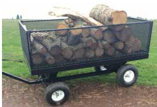
**Cart's front and rear axles pivot independently from side to side, thanks to Kuenzi's home-built suspension system.**
