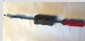
**James Nicholson, Lisbon, Ohio:** “I work on small engines and had need of a puller to remove an exhaust valve seat. I had recently been to a local garage sale and I purchased some small gear puller legs. I decided I could make a puller out of one. I cut one leg in half and welded it into a 3/8-in. threaded bolt coupler. Now it screws onto my seal puller and works great.”
