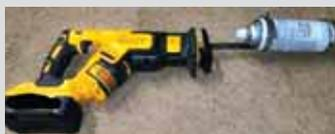
**Glenn A. Haley, Andover, N.H.:** “A quick and easy way to thoroughly shake a spray paint can is to attach it to the blade in a reciprocating saw. Just use a couple hose clamps to hold the can on the blade and insert
