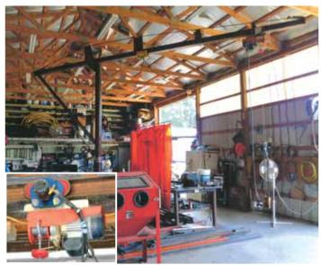
Overhead crane is located in center of Mariner's 30 by 60-ft. shop and can pivot 360 degrees to reach a pair of big doors spaced 30 ft. apart, as well as overhead storage shelves. Electric trolley and hoist run on a track made from a 15-ft. long beam.
