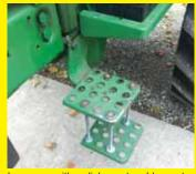
I came up with a slick way to add an extra step to my Deere 4230 tractor, attaching it to the tractor's original step with four threaded rods along with washers and nuts. I welded the washers on the top step to the top of the nuts so they lay flat on the step. By adjusting the threaded rods, I can easily adjust the distance between steps. (Timm Johnson, 1866 Knox Road 500 E., Galesburg, III. 61401 ph 309 343-6817; buzman5000@ yahoo.com)
