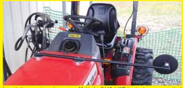
I needed a rear view mirror on my Mahindra 2415 4-WD tractor to use on roads. I couldn't justify spending a lot of money so I made a magnet-mounted bracket that attaches to the hood just ahead of the steering wheel.
