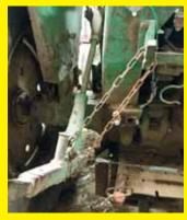
If your 3-pt. hitch "sags", making connecting the pto difficult, you can wrap a chain around it to keep it at the right height. (Fritz Groszkruger, Dumont, Iowa)
