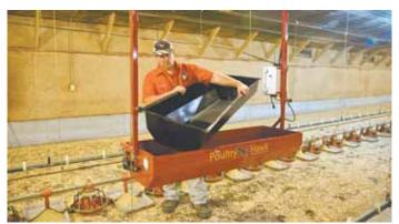
Poultry Hawk was developed to move dead birds out of poultry houses, but it's being used with feed trays, egg carts and even a sprayer for applying vaccines, insecticides
