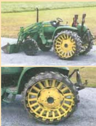
“Our new way of using rubber lugs on steel wheels offers a big improvement in both traction and comfort,” says Melvin Stoltzfus, J.S. Welding. “They provide the grip of an air-filled, lugged rear tire while maintaining a smoother ride.”
