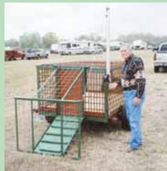
Harry Stracener’s 2-wheeled “transfer trailer” is equipped with a loading ramp on back that’s raised and lowered by cranking a hand winch.
