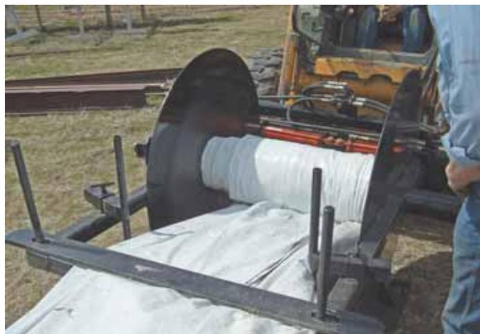
Hydraulic-operated unit rolls up empty silage bags into a tight coil secured with baler twine.
