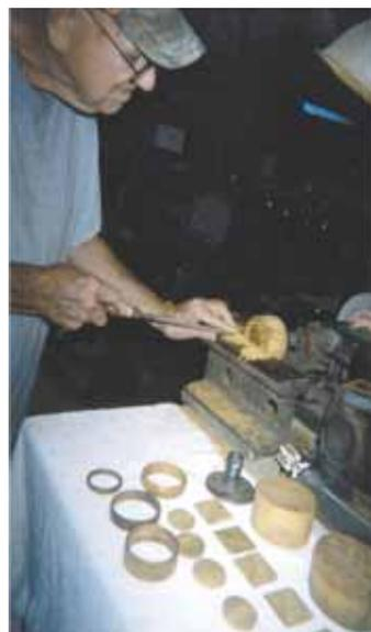
James White turned a grinder into a lathe by welding a nut onto the grinder shaft, and then screwing a 4-in. faceplate onto it.
